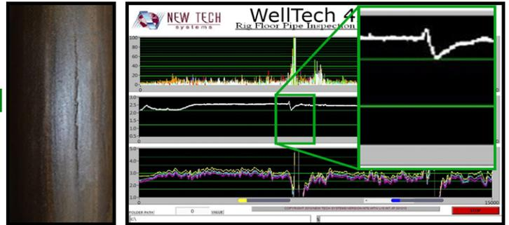
Left: Longitudinal Split In Tubing From Rod Wear
