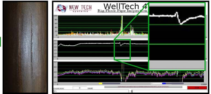
Left: Longitudinal Split In Tubing From Rod Wear Right: Split Detected With WellTech Software
